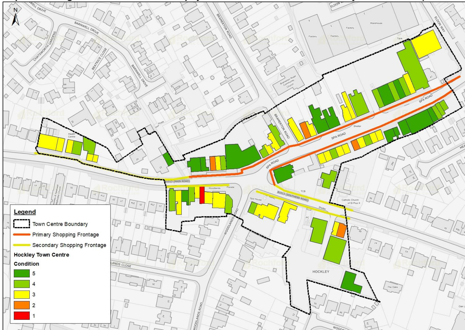
Figure 22 Map illustrating the classification of the physical condition of units in Hockley Town Centre (October 2023).
