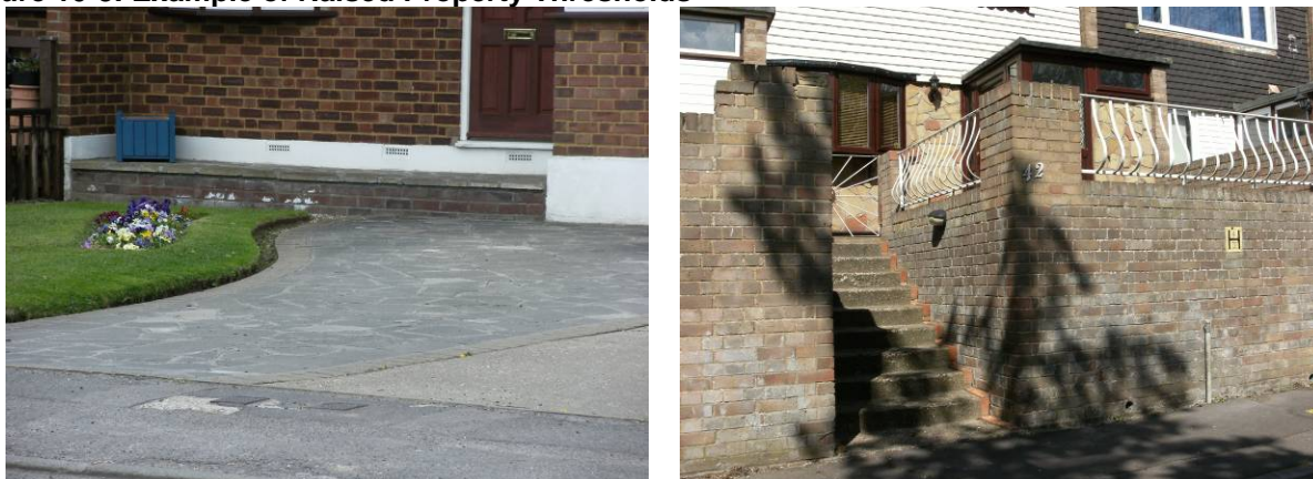
Figure 10-8: Example of Raised Property Thresholds
