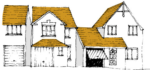
Integral garage doors can be unduly dominant and damage the scale
